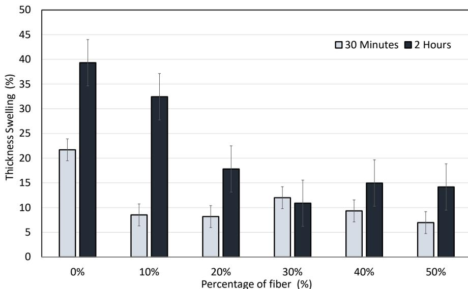
Figure 3. Thickness swelling results from TPCS reinforced with coconut fiber
