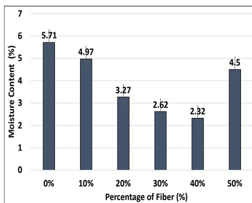
Figure 4. Moisture content results for TPCS reinforced with coconut fiber
