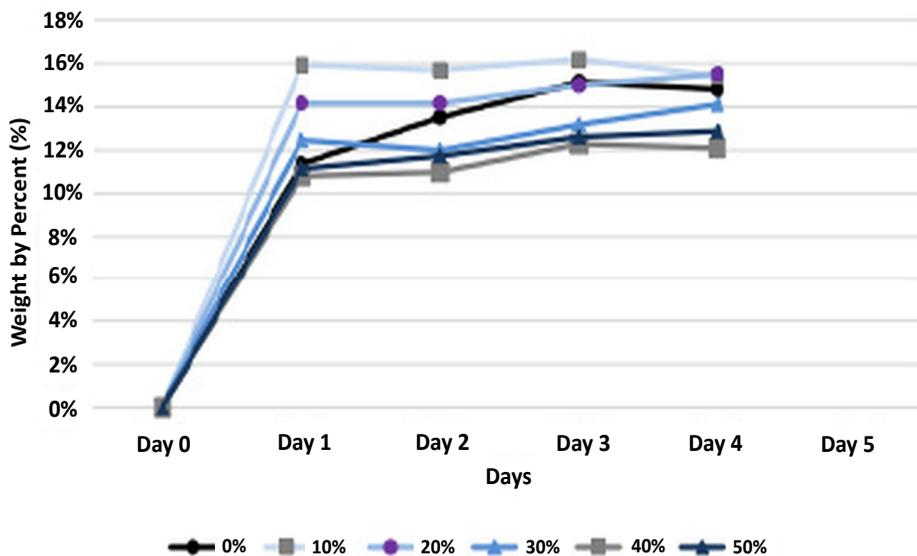
Figure 6. Moisture absorption of TPCS reinforced with coconut fiber
