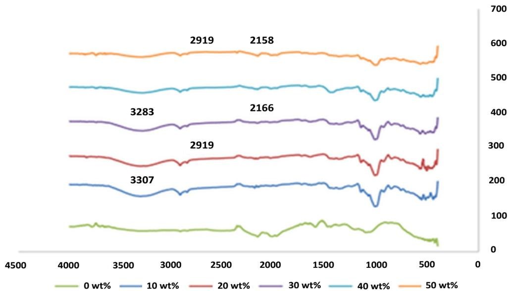
Figure 2. Results obtained from conducting the FTIR test on the TPCS reinforced with coconut fiber
