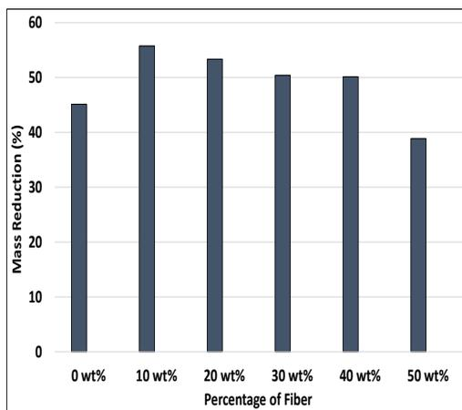
Figure 9. Mass reduction (%) from the soil burial test for TPCS reinforced with coconut fiber
