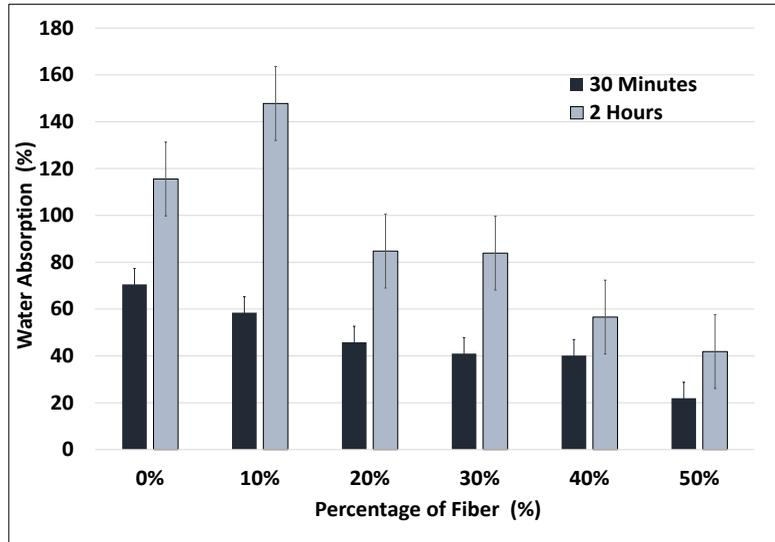
Figure 5. Water absorption result for TPCS reinforced with coconut fiber
