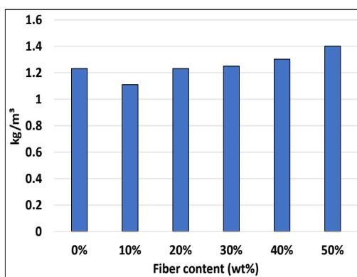
Figure 7. Density of TPCS reinforced with coconut fiber
